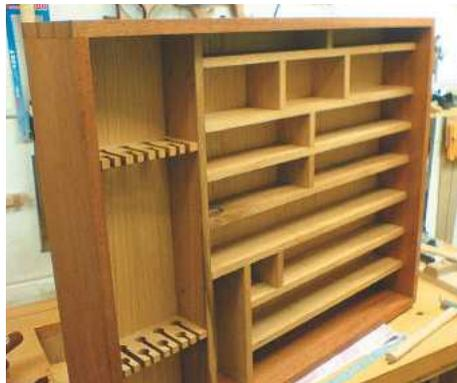
▲ Pic.18 The completed plane and chisel cabinet. Note the cut-outs for storing chisels
